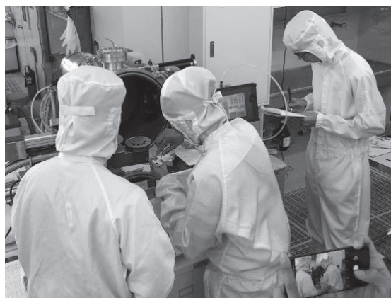
Fig. 1. Setting samples at the ion-beam etching equipment in the clean room.
